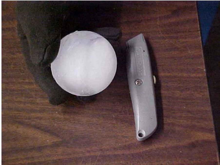
Photo 2: Sphere of frozen ice for impact testing
